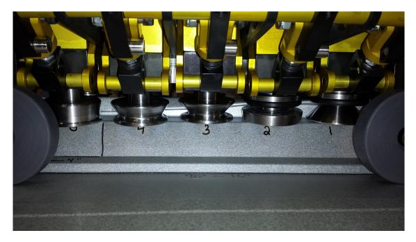
The seamer must be engaged in this manner. Failure to do so will result in panel damage.
